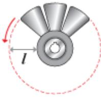
A turbine blade is subjected to huge centrifugal load, which will be one of our critical factors in selecting the material. The blades also must not fail due to bending during sudden turbine acceleration or vibrations. This requires high strength and resistance to brittle failure. The radius of the turbine (length of the blades,  $l$ ) will be determined mainly by flow and space considerations and is therefore treated as fixed.
