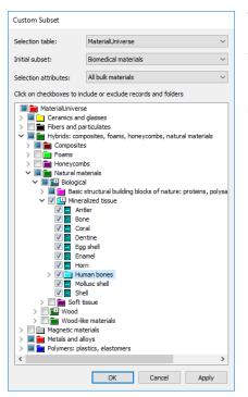
The Custom subset of *Biomedical materials* at Level 3 is modified by adding all *Mineralized tissue*. The *Human bones* records are changed to white and added to favourites by right-clicking. Since the stem cannot have a yield strength or elastic modulus lower than cortical bone, these constraints are added by a box selection, positioned so that materials with values above the *Femur cortical bone* properties are included. Fracture toughness and other constraints can be added in a Limit stage.
