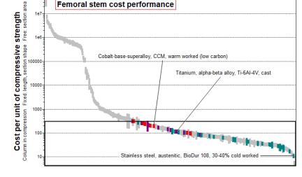
Cobalt chromium alloys are highly resistant to corrosion and have some mechanical properties that are superior to stainless steels, such as fracture and fatigue resistance. Although more expensive than these steels, cobalt chromium is still used for the ball joint of the head. It has, however, gradually been replaced by titanium for the stem part. Ti-6AI-4V osseointegrates and has:
