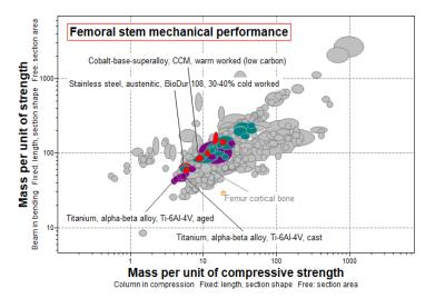
The way we screened for austenitic grades, was to filter on magnetic properties in the Limit stage. Non-magnetic grades were selected in the drop-down menu for *Magnetic type*. In implants, austenitic stainless steels are used, rather than martensitic, partly due to:
