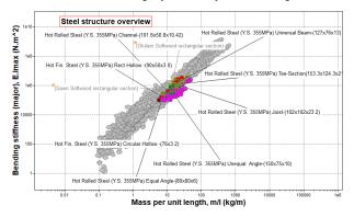
For these structures, low mass per unit length is more important than low density. Bending stiffness is maximized. We can see that steels occupy the middle range of the chart and that some woods, added for comparison, perform surprisingly well (basically planks of softwood or laminated beams, marked with stars).
