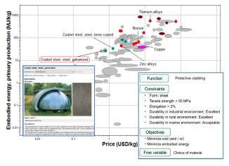
In this case, there is no mechanical performance to consider. The best materials can simply be identified in the chart after applying suitable constraints (see insert).
