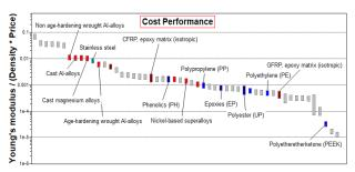
From this Bar chart, we can see that material cost considerations favour Al alloys Mg alloys and stainless steel over composites and polymers. It is likely, that this consideration greatly influenced currently used materials. In real chainsaw blades, the strength relies on structural design. There are several kinds of blades in real use which differ by internal structure, such as cavity filler, material combinations and the manufacturing processes
