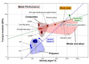
If index lines for maximization, with slopes 1 and 3, are added to the chart, just below the reference, materials that fall below this reference are screened out. If the
