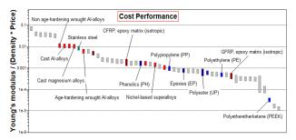
From this Bar chart, we can see that material cost considerations favour Al alloys, Mg alloys and stainless steel over composites and polymers. It is likely, that this consideration greatly influenced currently used materials. In real chainsaw blades, the strength relies on structural design. There are several kinds of blades in real use which differ by internal structure, such as cavity filler, material combinations and the manufacturing processes.
