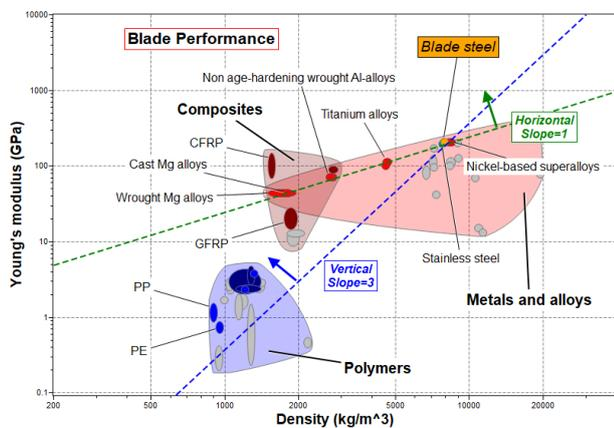
If index lines for maximization, with slopes 1 and 3, are added to the chart, just below the reference, materials that fall below this reference are screened out. If the
