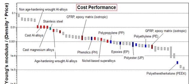
From this Bar chart, we can see that material cost considerations favour Al alloys Mg alloys and stainless steel over composites and polymers. It is likely, that this consideration greatly influenced currently used materials. In real chainsaw blades, the strength relies on structural design. There are several kinds of blades in real use which differ by internal structure, such as cavity filler, material combinations and the manufacturing processes
