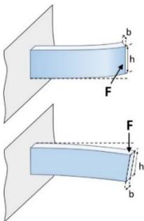
In GRANTA EduPack, the situation can be mechanically likened to a fixed-end beam loaded in bending by horizontal or vertical forces, as shown to the left. A translation of the problem involves specification of the *function*, *constraints* and the *objective* of the selection.
