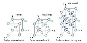
*Ferritic* stainless steels rely on *added Cr* and contain small amounts of C, usually less than 0.10%. These are the cheapest and are popular in, *e.g.*, cutlery. Mo can be added for aggressive conditions such as sea water. Ferritic stainless steels are ductile but not as formable as Austenitic.
