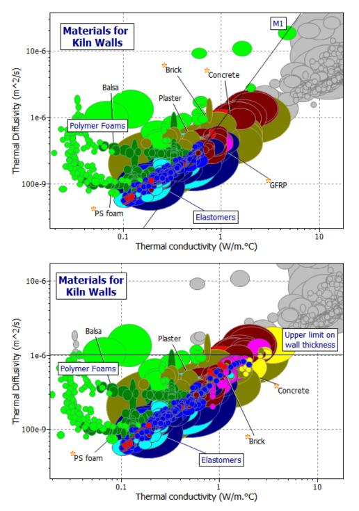
Figure 2-2. Thermal diffusivity, a , (a compound-property) plotted against thermal conductivity  $\lambda$  using the generic record subset. The selection line of slope 2 shows  $M_1$ ; materials above the line are the best choice, provided they lie within the thickness-limit (right-hand scale and horizontal broken line).
