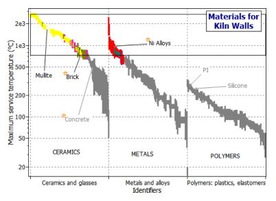
*Figure 2-4. Maximum service temperature plotted against material class. Only metals and ceramics can tolerate temperatures as high as 1000 K; metals are eliminated by their high thermal conductivities.*
