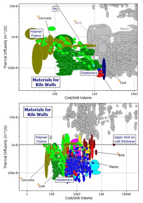
Figure 2-3. Thermal diffusivity, a , (a compound-property) plotted against cost per unit volume using the generic record subset. The selection line of slope -2 shows  $M_2$ ; materials below the line are the best choice, provided they lie within the thickness-limit (right-hand scale and horizontal broken line).
