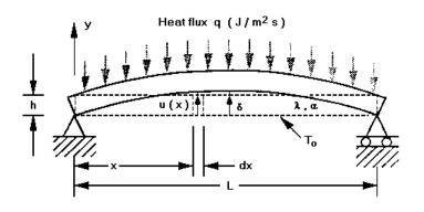
Figure 4-2. The distortion of a beam caused by a heat flux on one of its faces.
