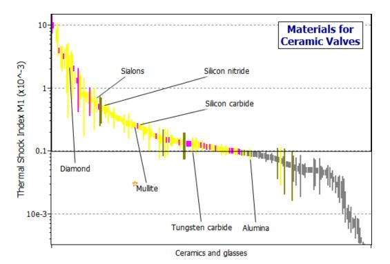
*Figure 5-2.* The index describing thermal shock resistance of ceramics. The horizontal line passes through alumina.
