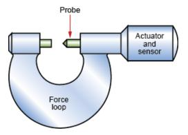
*Figure 4-1. A precision device. All such devices have a force loop ; the precision depends on its dimensional stability.*
