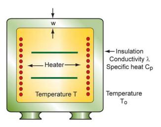
*Figure 2-1.* A kiln. In a firing cycle, energy is lost both by conduction and in heating the structure of the kiln itself.
