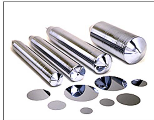
Device grade silicon boules and wafers. (Image courtesy of <http://www.chipsetc.com/silicon-wafers.html>)
