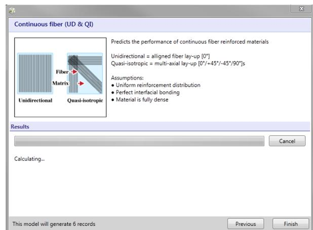
Recall that our simple model is calculating density and Young's modulus for a hybrid material using the rule of mixtures:
