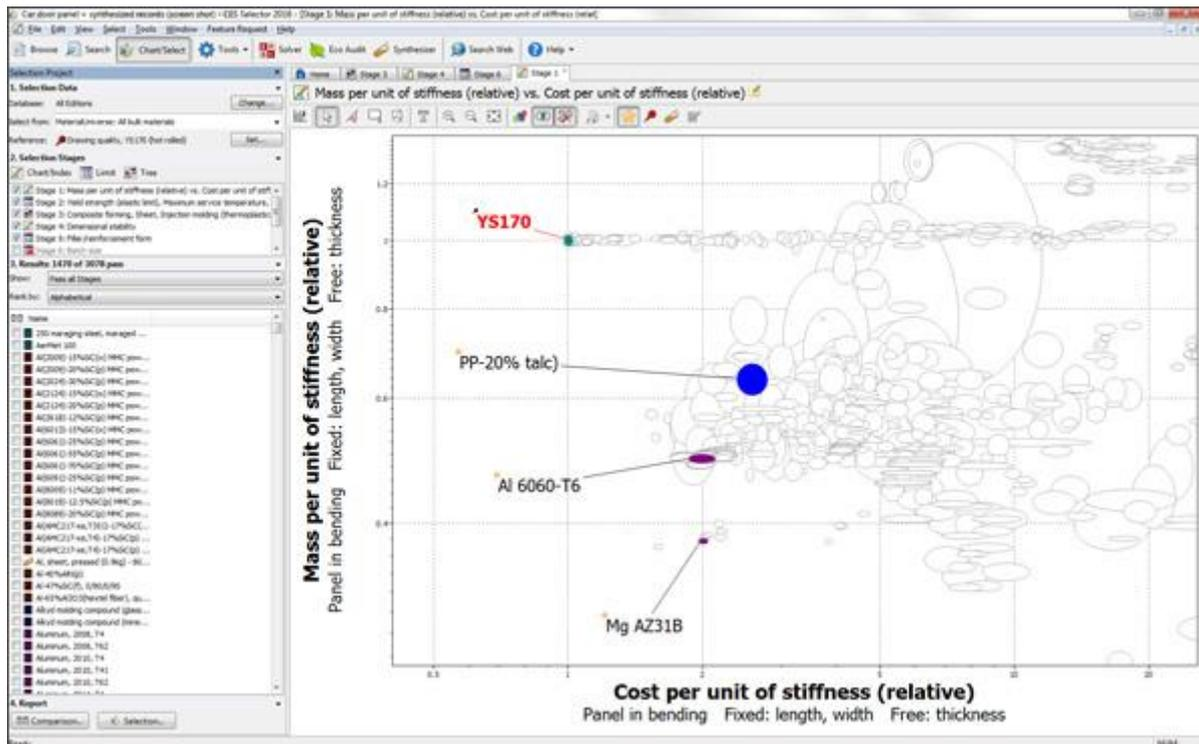
The chart shows that the polypropylene could lead to a weight saving of 35% relative to the steel, but at substantially higher (2.5 times) cost. However, this cost is based on just the material prices and does not account for processing costs. We can account for processing using the Part Cost Estimator model in CES Selector.
