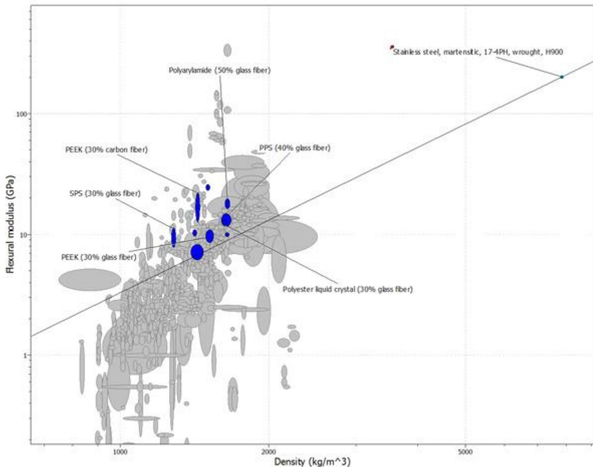
Figure 1: Stiffness-limited selection, minimizing mass : the line represents points with the same value of performance index. The highlighted materials are valid alternatives to steel 17-4PH.
