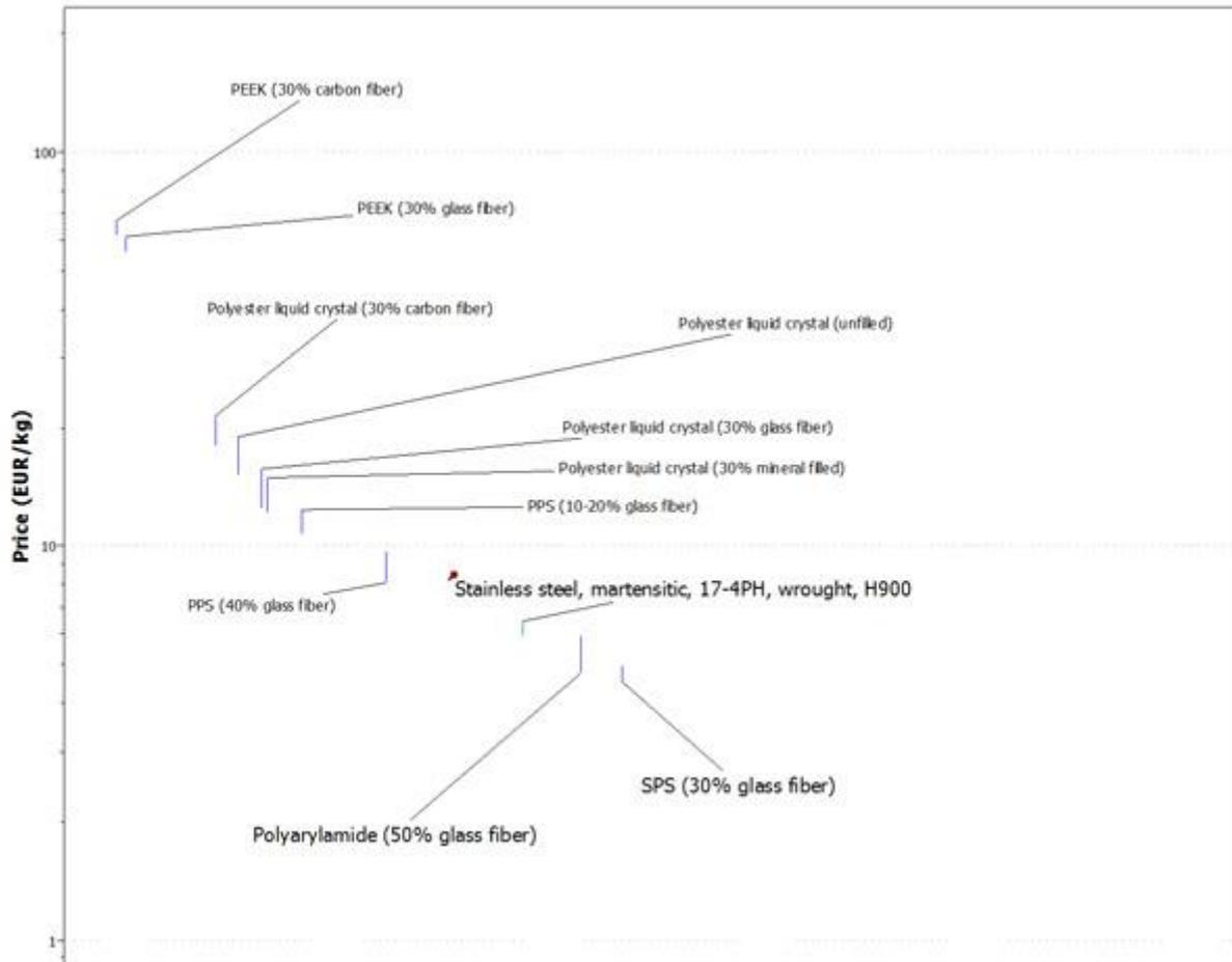
Figure 3: Cost ranking: the materials with a specific cost (i.e., cost per unit of mass) less than that of steel are PARA + 50% GF and SPS + 30% GF.
