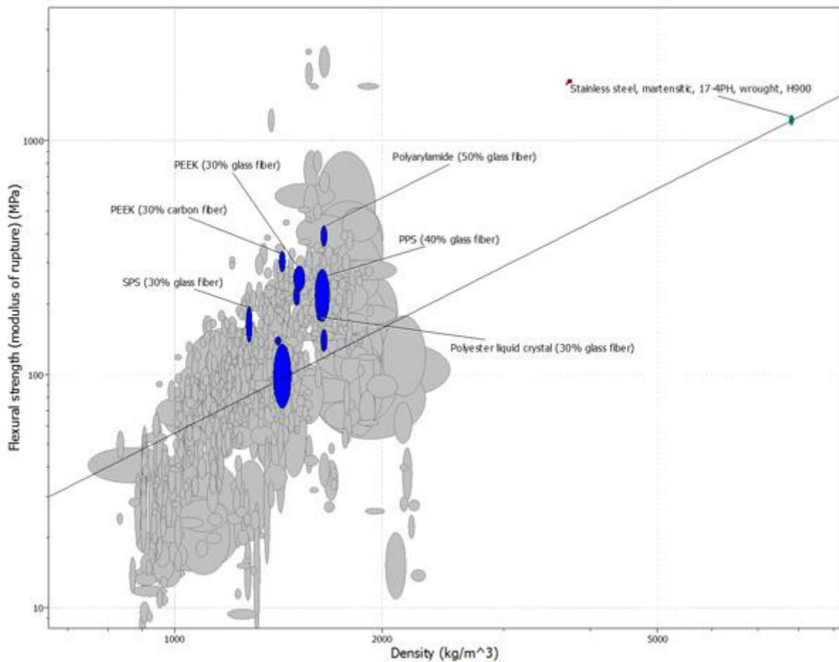
Figure 2: Strength-limited selection, minimizing mass: the line represents points with the same value of performance index. The highlighted materials are valid alternatives to steel 17-4PH.
